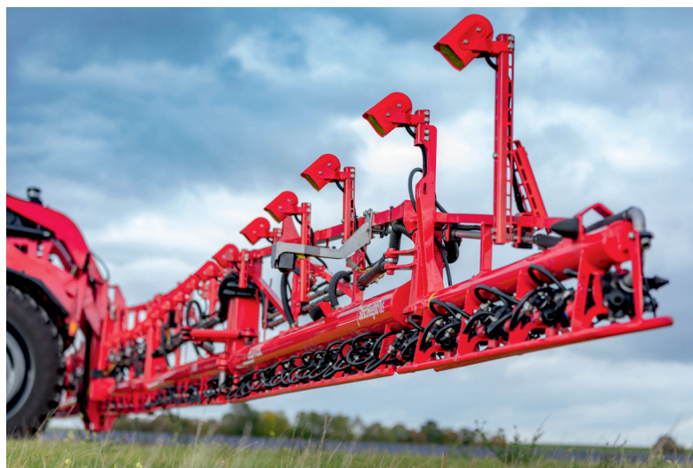
Fot. 3. Opryskiwacz samojezdny firmy Agrifac z zamontowanym systemem wizyjnym 3S Spray Spot Sensor® Photo 3. The self-propelled sprayer by Agrifac equipped with the 3S Spray Spot Sensor® vision system mounted
